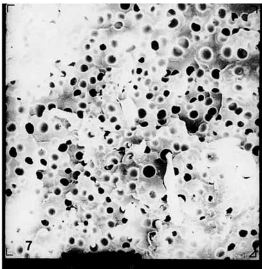
Figure 7 PMMA/PEO (70/30) without copolymer ( \times 1000 ).
