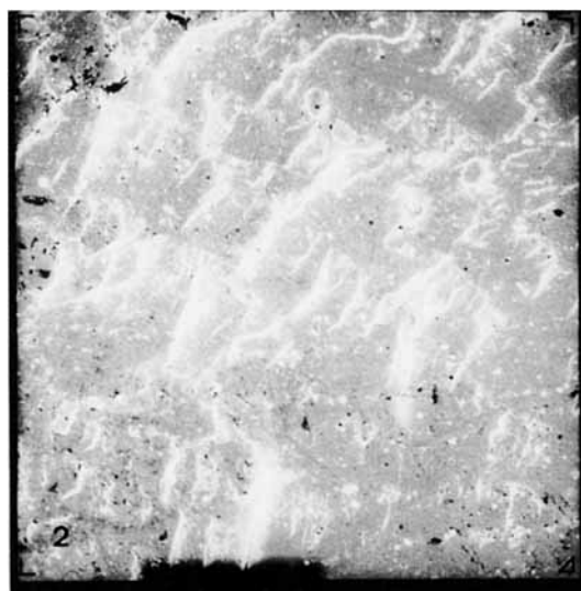
Figure 2 PMMA after treatment with methanol ( \times 1000 ).
